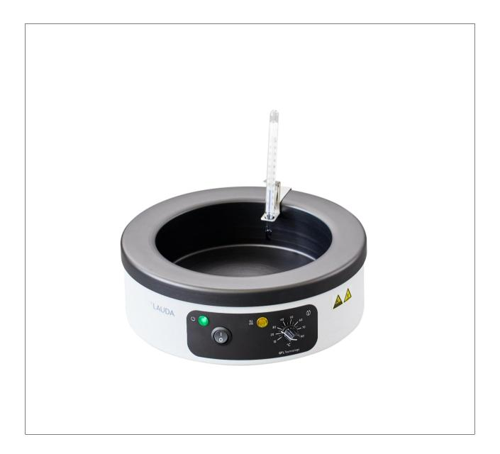
The LAUDA Hydro Tissue Float Bath H 2 P is a special bath for histological, pathological, clinical and bacteriological laboratories, for stretching and drying of cut tissue samples. The outer housing is made of powder coated aluminium, the bath body as well as the rims of the bath to dry the cut tissues are made of black anodised aluminium.
