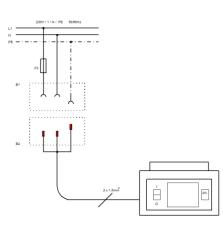
H 2 P for 230 V with power supply 230 V / N / PE / 50/60 Hz, connected through 3-pole shock-proof (Schuko) plug system.
